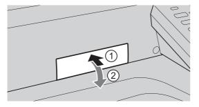
Insert a PCMCIA/PC Card Adapter into the PCMCIA/PC Card Slot as illustrated. (Label side up)
